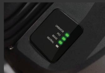
Our newest feature, Crank Assist, safely takes you step-by-step through the tractor's start-up process.
