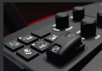
On cab models, the electronic rear hitch controls improve chore efficiency and overall productivity. Easily adjust lift speed, draft, depth, auto-raise on turns, & more.
