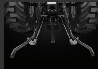
Our 3-point CAT 1 hitch has lift arm telescoping stabilizers for fast and easy implement hookup.
