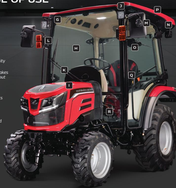
The Mahindra 2100 Series ROPS cab (Rollover Protection Structure) is designed, fabricated, and fitted at our assembly plant. It offers a comfortable ride all year round with built-in heat and air conditioning. Additionally, the glass-enclosed cab provides a 360-degree view and includes work lights, mirrors, and wipers to deliver an exceptional experience, setting a new class standard.
