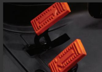
Our hydrostatic drive system (HST) eliminates gear-shifting by safely engaging color-coded forward or reverse pedals. Combining HST with super-smooth joystick control makes front loader work fast and efficient.
