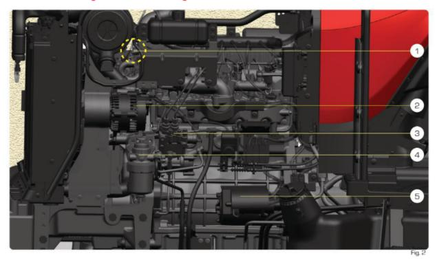
Left hand side view : 1. EGR cooler 2. Alternator 3. Fuel injection pump 4. Fuel filter 5. Starter motor
