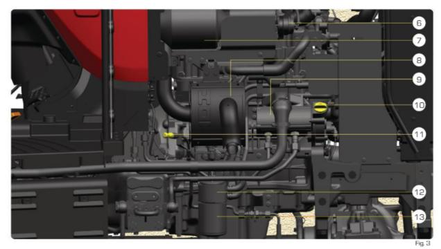
Right hand side view: 6. Turbo charger (55Hp) 7. DOC 8. Muffler (UHM) 9. Hydraulic tandem pump 10. Engine oil filling cap 11. Engine oil dipstick 12. Engine oil cooler (55Hp) 13. Engine oil filter
