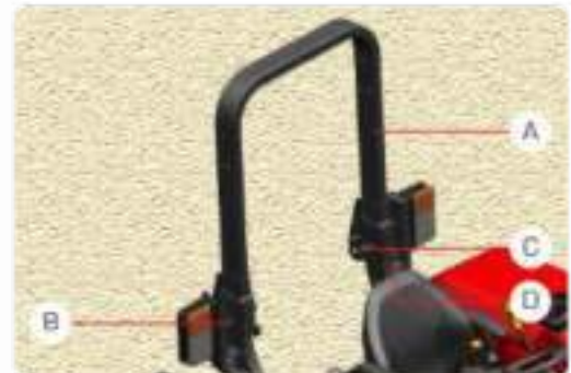
A - ROPS crossbar B - Quick-lock pins C - Headed pins D - Knob
