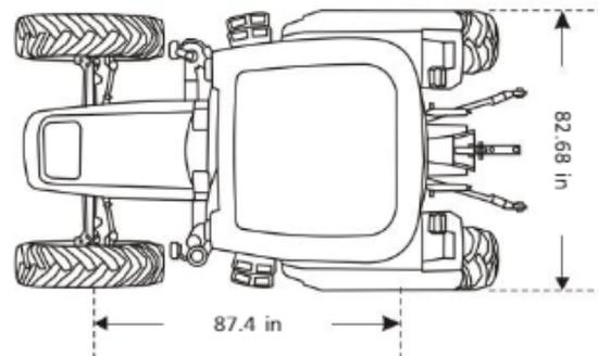
Dimensions are in inch. and based on 11.2 x 24 front tires and 16.9 x 30 rear tires.
