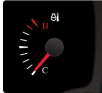
1. Indicates the engine coolant temperature is going to exceed the limit.
