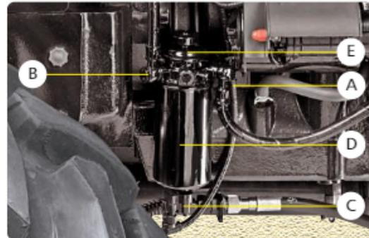
**NOTE :** Drain water once in a week or whenever the water level indicator on dashboard glows "ON" continuously, if water contamination is excessive. Continued driving with water accumulation in fuel filter will cause damage to the fuel pump / other fuel system components.
