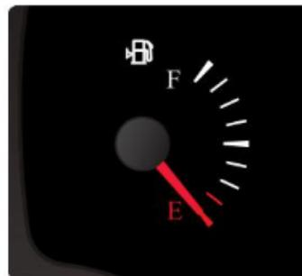
Low fuel indication & buzzer ON at 2<sup>nd</sup> Graduation & OFF at 3<sup>rd</sup> Graduation. Buzzer sound at the rate of 15 beeps per min.
