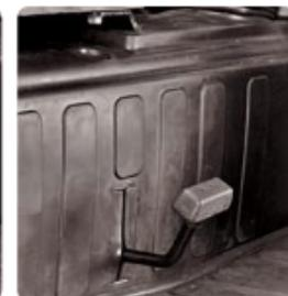
4WD Lever Disengaged
