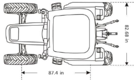
Dimensions are in inch. and based on 11.2 x 24 front tires and 16.9 x 28 rear tires.
