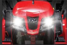
Using projector-style headlights for best-in-class output, we offer 8000 lumens of bright, white lighting for after-dark chores.
