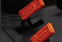
Our hydrostatic drive system (HST) eliminates gear shifting by safely engaging color-coded forward or reverse pedals. Plus. the tractor automatically slows down when releasing either pedal.
