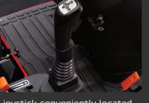
A joystick conveniently located next to the steering wheel controls our front loader. It's super smooth to operate, even for those with arthritis. Coupling this with our gearless forward and reverse pedals facilitates fast and efficient loader work.
