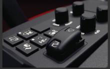
For Cab models: While others use levers, we switched to electronic 3-point hitch controls to improve chore efficiency and overall productivity. Now, it's easy to adjust lift speed, draft, depth, auto-raise on turns, & more.
