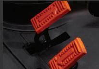
Our hydrostatic drive system (HST) eliminates gear shifting by safely engaging color-coded forward or reverse pedals. Combining HST with a suoper smooth joystick for loadercontrol makes fast and efficient loader work.
