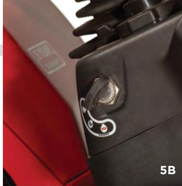
**SIDE IGNITION** Tractor operators are prone to knee-bumping their keys on front-facing ignitions. We addressed the problem with a simple solution, moving ours (5B) to the side.
