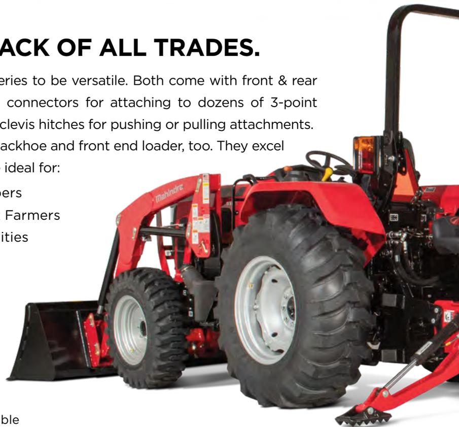
**VERSATILE 3-POINT HITCH** You'll be able to connect to dozens of implements and take on any task with our ball-pivot CAT I (8A) & CAT II (8B) connectors with telescopic stabilizers & flex links.
