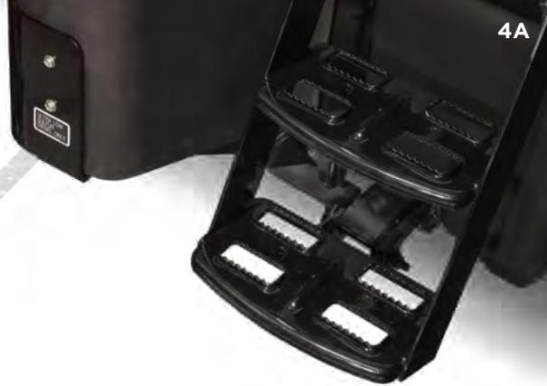
**EASY ENTRY** We added a two-step ladder (4A) for smaller operators. And we cleared the floor path so getting in and out of the tractor is a cinch.
