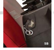
**SIDE IGNITION** Tractor operators are prone to knee-bumping their keys on front-facing ignitions. We addressed the problem with a simple solution, moving ours (5B) to the side.
