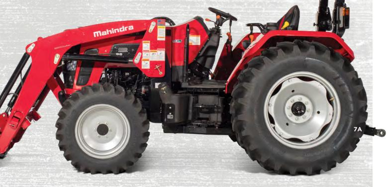
**HEAVY-DUTY, HEAVY-WEIGHT** Our base model, with agriculture or industrial tires, is rock-solid at 5390 lb. Attach a front loader, and this 6,690 lb 4WD tractor becomes an unstoppable beast.
