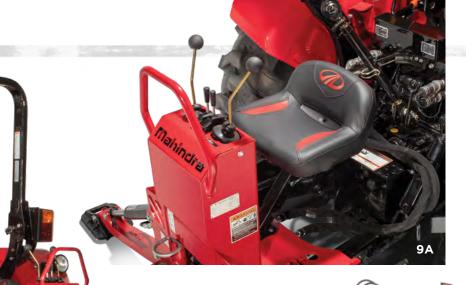
**BACKHOE OPERATOR STATION No** more awkward turning from the driver's seat. Instead, we've added a relaxing forward-facing station (9A) that puts you in absolute control of your bucket list.
