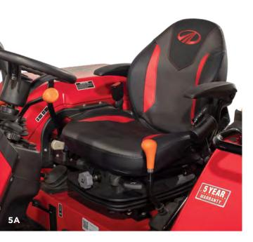
mCOMFORT SEAT First, we didn't skimp by using a lawnmower seat. Nor did we ignore details like tractor vibration. Instead, we created the industry's most innovative chair (5A) ever, including contoured lower and upper seat cushions, integrated armrests, and forward and backward adjustable legroom. Plus, it comes with a soft-coil suspension to help prevent fatigue on those long days and a retractable seatbelt for added safety.
