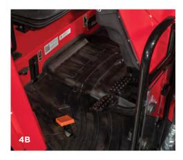
NEAR-FLAT PLATFORM We engineered our operator platform (4B) with the lowest hump possible. Our near-flat floor reduces the tripping hazard and provides maximum real estate for your feet when seated. Our tractor comes with an anti-slip rubber floor mat — standard — too.
