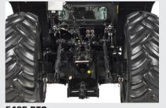
**540E PTO** Standard economy settings allow for less fuel consumption and lower noise levels in light PTO work.
