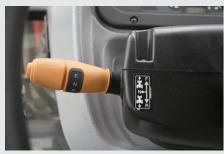
**PST TRANSMISSION** Standard 15x15 Power Shuttle allows for a wide speed range and excellent directional control for heavy-duty loader work
