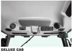
Each 6000 series model is available with a deluxe cab, fully equipped with air-conditioning, heater, a spacious interior, window wipers, flat deck ergonomic operator platform, and more.
