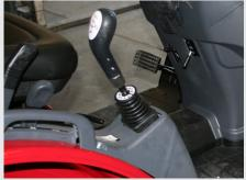
**LOADER OPERATION** Fender-mounted loader joystick makes loader operation easy and comfortable.
