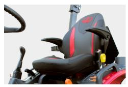
**WORK IN COMFORT** Mahindra's own mComfort seat is built for maximum ergonomic support. Features include extra cushioning for operator comfort, air suspension seats, and foldable armrests.
