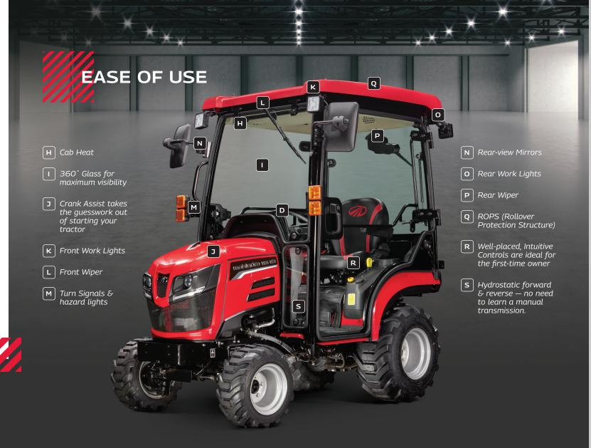
Mahindra 1100 Series ROPS (Rollover Protection Structure) cabs are engineered, manufactured, and installed on our assembly line. And it can be easily heated for ultimate comfort on those blistering cold days. Moreover, our glass-surround cabs have a 360° field of view and come with work lights, mirrors, and wipers for an overall best-in-class experience.
